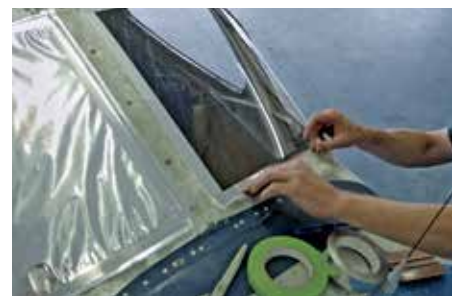
Plane paint masking
