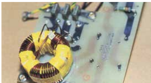
Coil outer wrap taping
