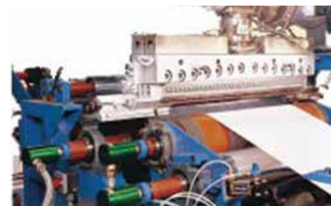
Orange overcoat masking tape on chill roll
