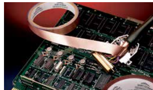
EMI-RFI copper tape shielding
